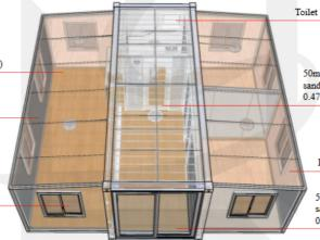
50mm EPS sandwich panel/rock wool sandwich panel, 0.326 / 0.376 / 0.426 / 0.476mm steel plate
